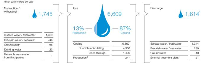
The difference between the volume of water drawn and the volume discharged is primarily attributable to evaporation losses during closed-circuit cooling.
